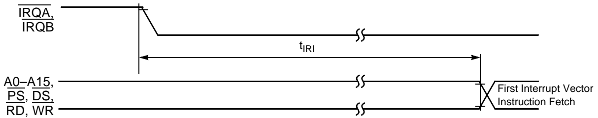
Figure 3-15 Interrupt from Wait State Timing
